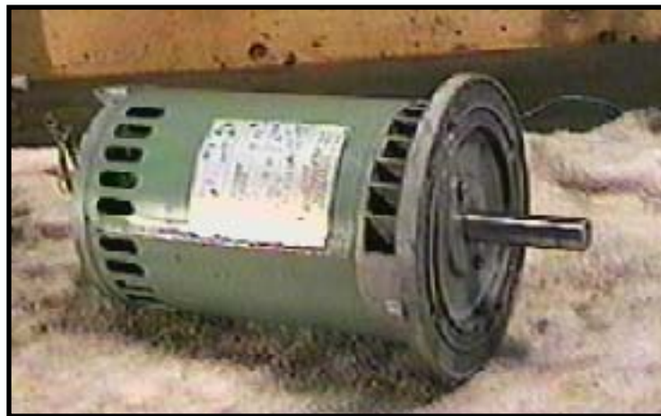
Typical waterpump motor
