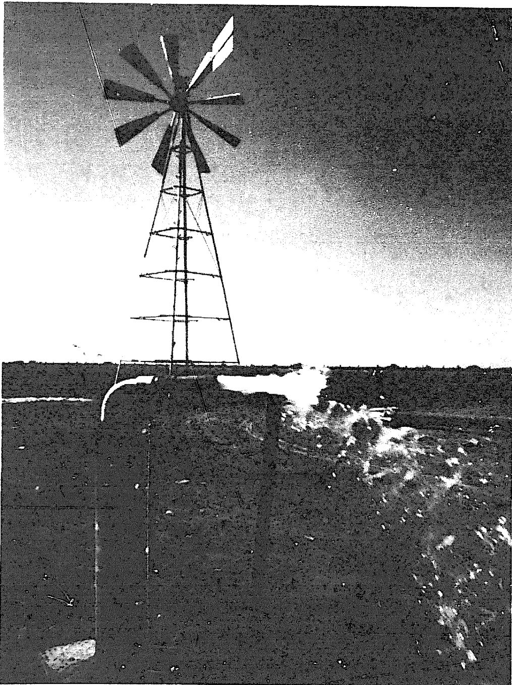
At times the value of water is incalculable. A Mapel compressor windmill pumping from 80 meters by the air lift principle during a drought in the Northeast of Brazil.
